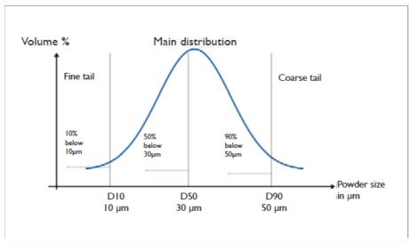
Figure 5: Example of D10, D50 and D90 on a PSD curve for a 10-50 microns powder
