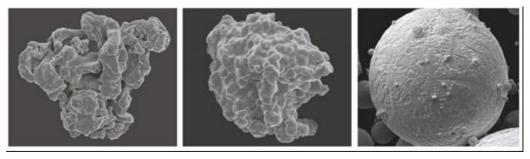
Figure 4: Examples of powders with different morphologies. [8]
