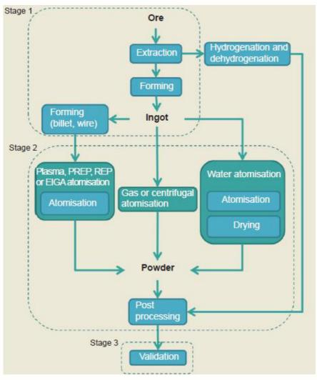
Figure 3. Powder production steps flow chart from ore to validated AM powder [6]
